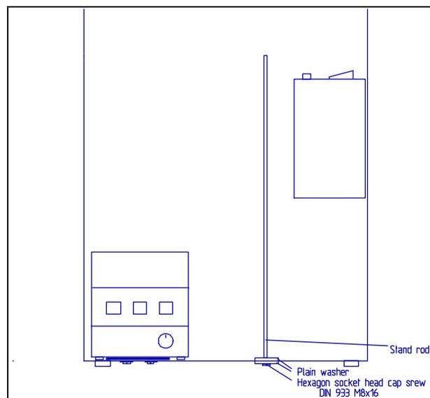
Pullout the stirrer cable from the bottom of the stirrer. Slide the photometer over the stand rod and fasten it. Then slide the flask holder, the clamp ring and the electrode holder over the stand rod.
