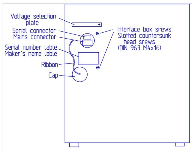
Check if the voltage selection label at the rear of the case matches your mains supply voltage. If the voltage is not correct open the interface box by the four screws at the front and switch the voltage selector to the desired position. To change the voltage selection of the Dosimat see the Technical Reference Manual, page 13. Don't forget to turn over the voltage selection label at the rear of the case to ensure that the label indicates the current settings.
